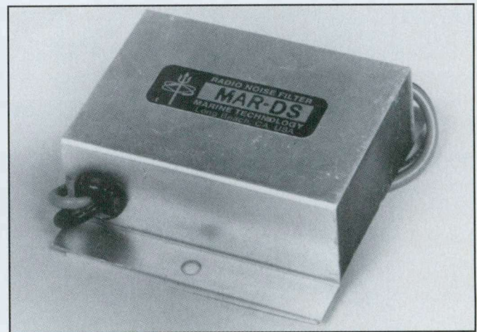
Noise filters will help minimize noise from inverters.
