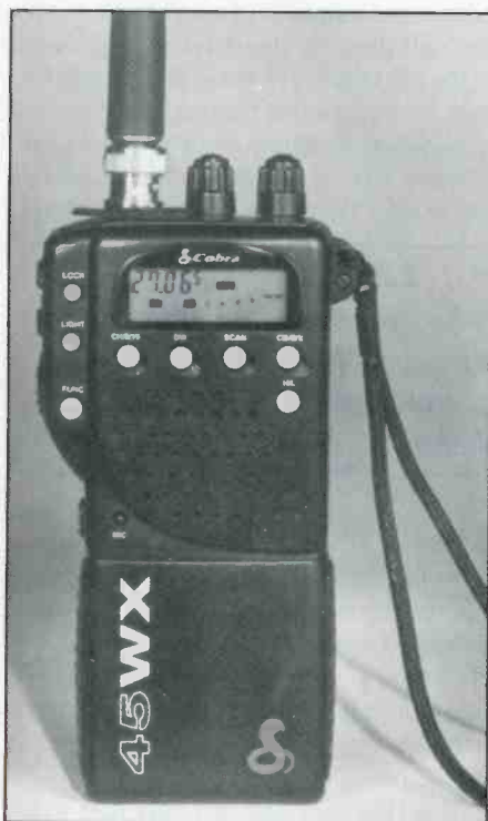
Cobra's diminutive HH-45WX is loaded with sophisticated features, including 10 weather channels, scanning, dual watch, 40 AM channels, plus lots more.
