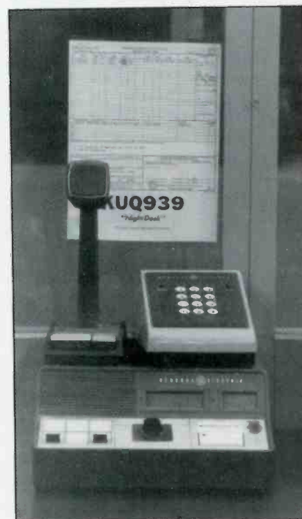
This is the dispatch remote and paging encoder used for dispatching reporters and photographers at a New Jersey newspaper. (Photo by Chuck Gysi, N2DUP)
