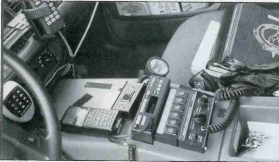
The console of my police cruiser features a 100-channel Bearcat Sportcat (with a mag-mount antenna on top of the cruiser for better reception), Motorola Spectra 800 MHz police transceiver, and a Tandy handheld cell phone. A CB radio is not visible in the photo, but I keep an ear on Channels 9 and 19. (Photo by Eric Jagoe)
