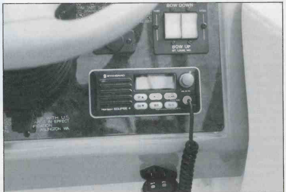
A 25-watt VHF transceiver can be found for under $139! This is Standard's "Horizon Eclipse +" transceiver.
